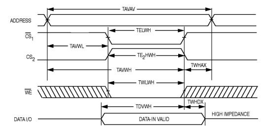
Note: The internal write time of the memory is defined by the overlap of  $\overline{CS1}$  Low and  $\overline{CS2}$  HIGH and  $\overline{W}$  LOW. Both signals must be actived to initiate a write and either signal can terminate a write by going in actived. The data input setup and hold timing should be referenced to the actived edge of the signal that terminates the write. Data out is high impedance if  $\overline{OE} = V_{IH}$ .
